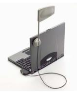
AnalyzeAir software interprets the RF energy in the spectrum or channel and lists the devices that are transmitting – associating real devices with the energy pulses. It automatically identifies Bluetooth® devices, cordless phones, microwave ovens, analog video cameras, and RF iammers. Then the "Device"
